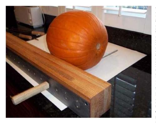
To drill parallel holes for the axles, place the pumpkin next to the jig. Hold the pumpkin firmly in place and punch the first axle hole by pushing the steel rod or drilling with along 5/16" bit. Insert a 5/16" rod through the jig into the pumpkin to stabilize it in order to make a second axle hole and repeat the punching/drilling process.
