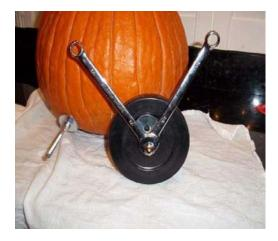
It is important that after the lock nuts are tightened there is enough room for the wheels to rotate freely, but not so much room that they wobble. To avoid this problem, insert a fender washer between the wheel and lock nut as shown in the photo on the right.
